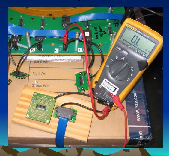
After confirming that everything is connected as shown above, move the female end of the blue test cable from the shorting plug to the test connector. As shown in the next image
