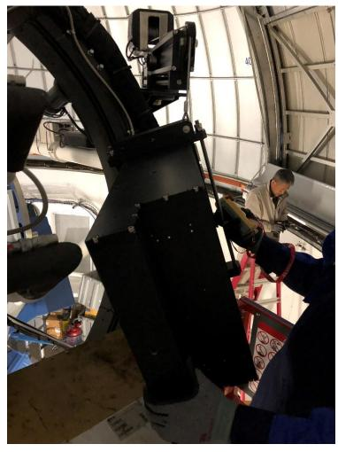
13. Put the FSA on the scissor lift
